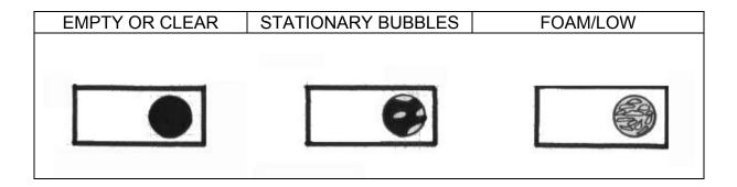
6.Feel the SEA FROST Plate in the icebox five minutes after engaging the timer switch. If the sight glass clears yet the plate temperature does not drop after **5** minutes of operation, turn off the system and CALL US AT **603-868-5720**.
